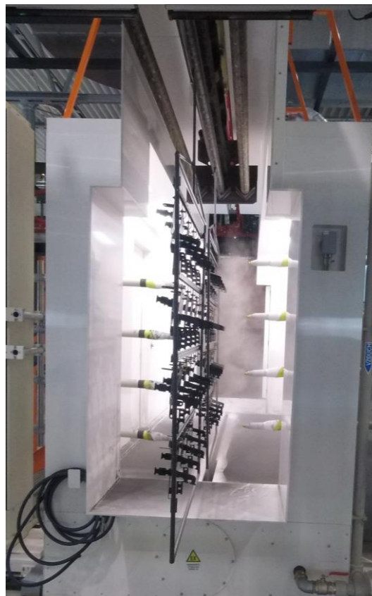
Powder Painting being done in fully automatic powder cabin
